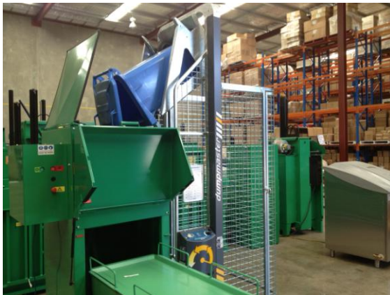
Glass Crusher (23 seconds per bin load)
